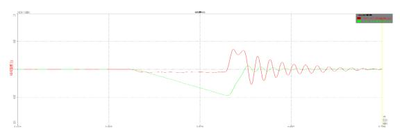
(2) Test once with the rated speed 0.50 m/s, rated load 1500 kg, system mass 6700 kg.
