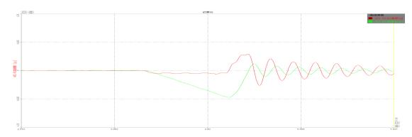
(3) Test once with the rated speed 3.0 m/s, rated load 1500 kg, system mass 6700 kg.
